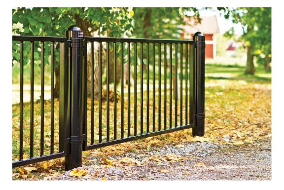
Fencing for greater enjoyment and safety. Flexible wrought iron fence with vertical square bars, height 900 mm (c-c 2000 mm). Complete sections are affixed to the posts with a clamping ring and can therefore be turned to the desired angle. To create some differences in level, the sections may be stepped. The images show the first section.
