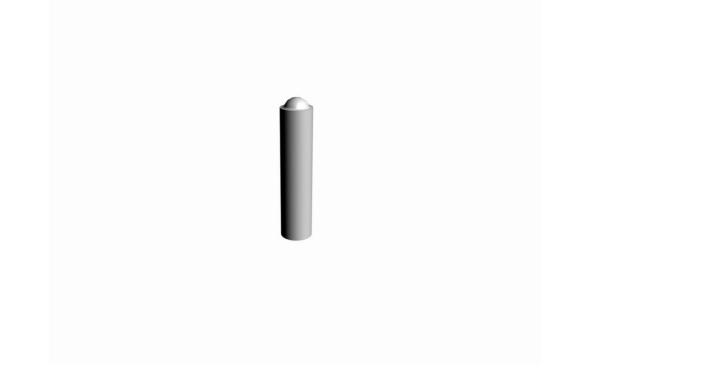
Bollards for roads and public squares. Cylindrical bollards for communal areas where pedestrians and drivers share the same space. The bollard is steel, 750 mm high and c-c 220 mm. Designed for poured foundations.
