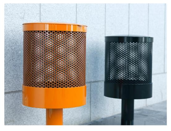
Medium-sized litter bin with lid. William is a medium-sized litter bin with a tight-fitting lid. This 55-litre bin is made from 3 mm powder-coated steel. For fixing, the litter bin is set in poured foundations with the accompanying central post (108 mm) or with the fixing plate.
