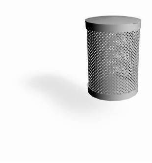
Litter bin with lid. Reuben is a litter bin made from 3 mm powder-coated steel, and has a tight-fitting lid. The bin has a volume of 35 litres and can either have poured foundations with a central post (40 mm)(NF2465), or be fixed to the wall or fitted on an existing post (105-120 mm)(NF2467).
