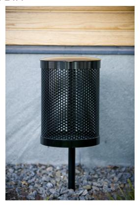
Litter bin with lid. Ruben is a litter bin made from 3 mm powder-coated steel, and has a tight-fitting lid. The bin has a volume of 35 litres and can either have poured foundations with a central post (40 mm), or be fixed to the wall or fitted on an existing post (105-120 mm).
