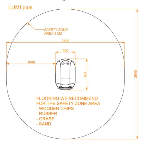
Rocking equipment "LUMI PLUS", model: 2016 01, designed according to the requirements of EN 1176 – 1:2017 and EN 1176 – 6:2017, is children's rocking equipment with support at one point and movement in many directions. Support - steel coil spring operating on tension and compression.
