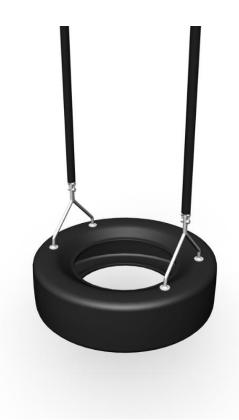
The length of the chains is about 160 cm. The swing seat is suitable for the following swings: 220001M, 220002M, 137414M, 137412M, 137418M, 175074, 175075, 220061M and 230050. The material of the chains is polished austenitic stainless steel, 6 mm thick. The chains have plastic coatings that protect the child. The seat is made of rubber.
